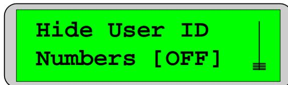
Press **Enter** to change the setting. You will be presented with a screen that accepts a **1** key to turn the star characters On (hiding the numbers) or a **0** key to turn the star characters Off (revealing the numbers). You do not need to press Enter again. As soon as you press 1 or 0, the value is set.
