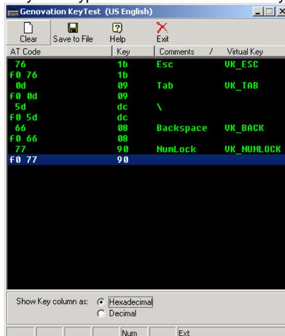
Type on your ControlPad. You should see the data that is programmed into the keypad appearing in the KeyTest panel. Click on **Exit** to close KeyTest when you are finished with it.
