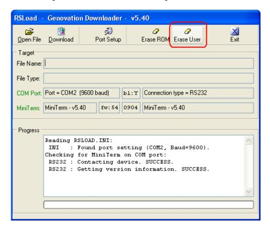
You can perform the above procedure using RS-232 or USB. For the actual firmware upgrade you will need to use RS-232.
