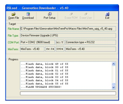
After the upgrade the MiniTerm will reboot. You can confirm the upgrade by clicking on **Port Settings** followed by **Ping MiniTerm**. Again the MiniTerm will be interrogated for its version information.
