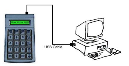
If you are hooking the MIDI Patch Changer keypad to a **PC that has USB**, then you can use the supplied RJ-to-USB cable:
