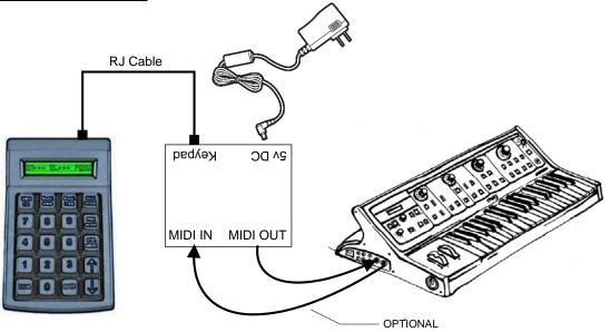
If you need to connect to **5-pin DIN MIDI** gear, then use the supplied Cat5 cable and supplied MIDI adapter box.
